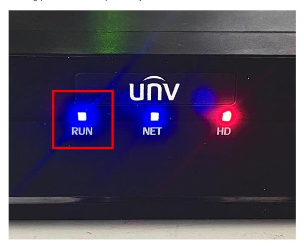
**Step 2** Unplug all the HDDs and Ethernet cables on the NVR, and let it run individually, then check if the NVR can boot up.
